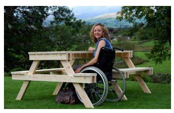
Fig.99 Example of a universally accessible picnic table
