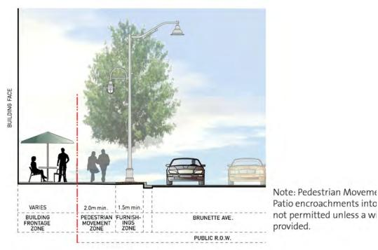
Figure-8 Type 'B' Cross-Section
